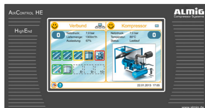
The ALMiG Air Control HE controls two compressors in combination. This allows the energy advantages of speed control to be fully exploited.
